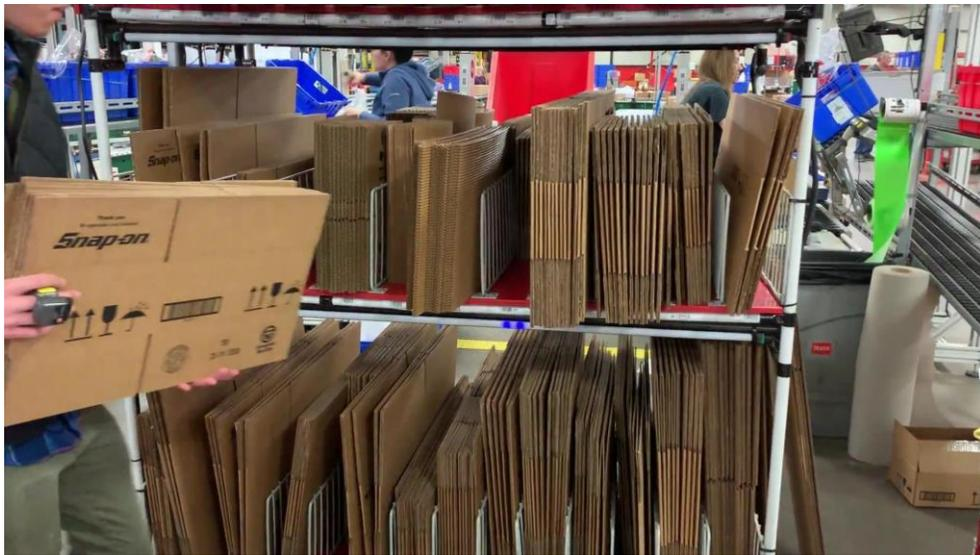
Fig. 6. Worker Inserts Replenishment Carton into Location Highlighted by LED Strip Segment
