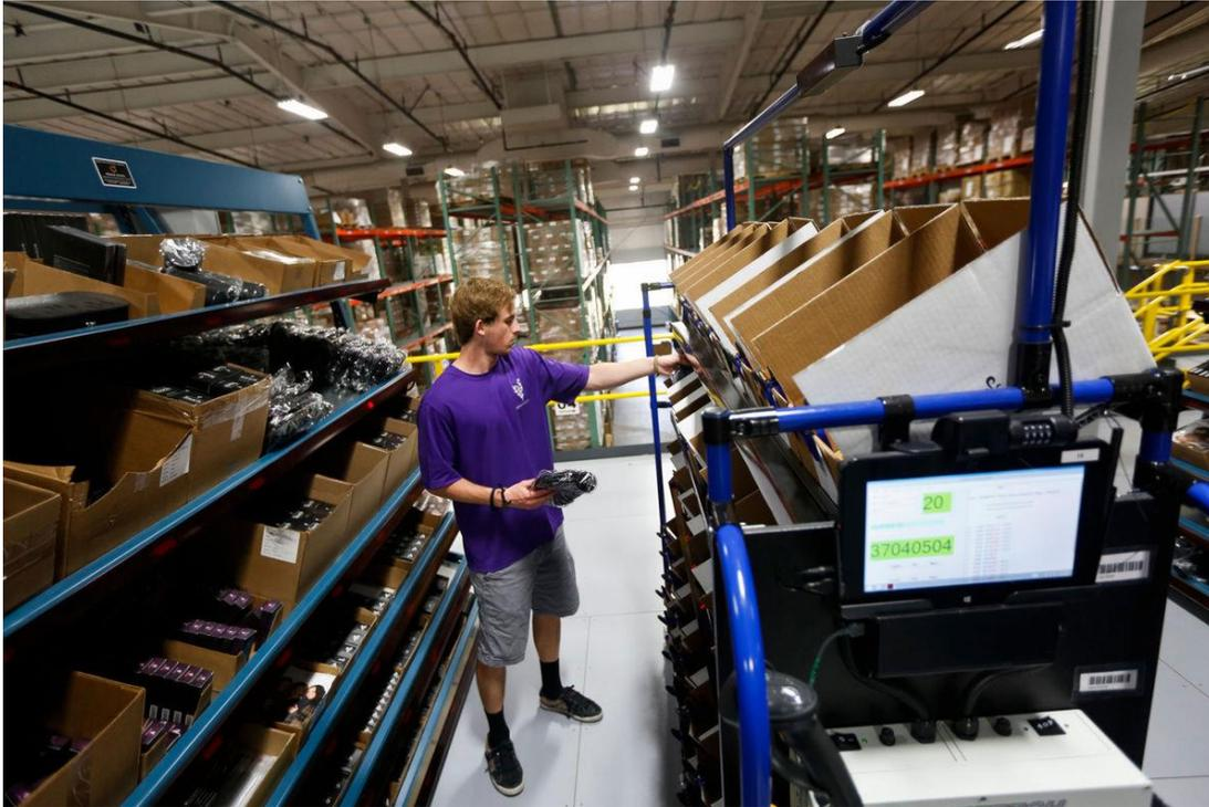
**Fig. 2** Multimodal Cart Used with Bays Having Numerical Displays Adjacent to Product Locations
