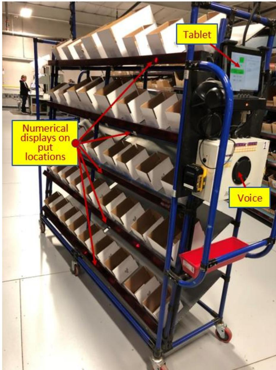
**Fig. 1** Batch-Picking Cart for Multimodal Order Fulfillment
